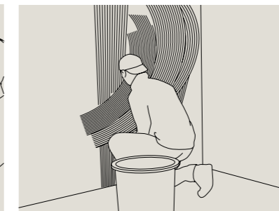
Application of Adhesive on the Existing Substrate
